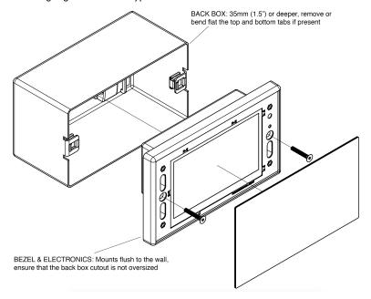
Carefully remove the protective films from the front of the liquid crystal display and the magnetic overlay before final assembly.
